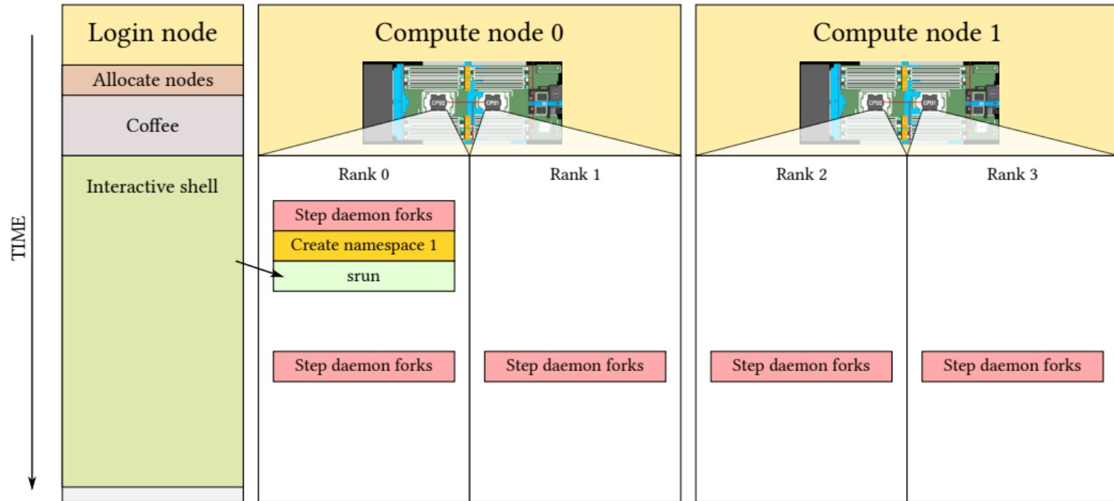
SLURM will fork a step process **outside** the safe environment.
