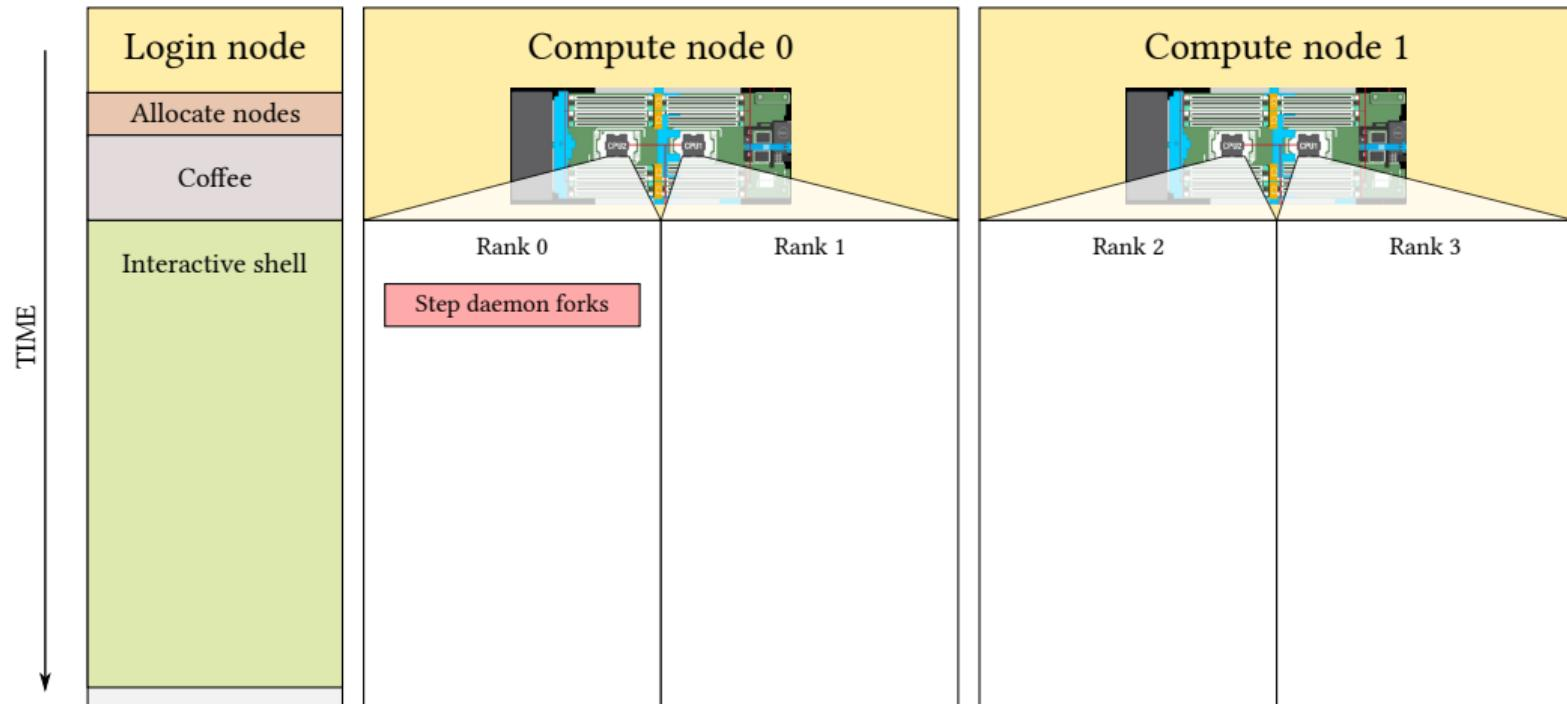
SLURM will allocate the nodes and fork a process in the first rank.
