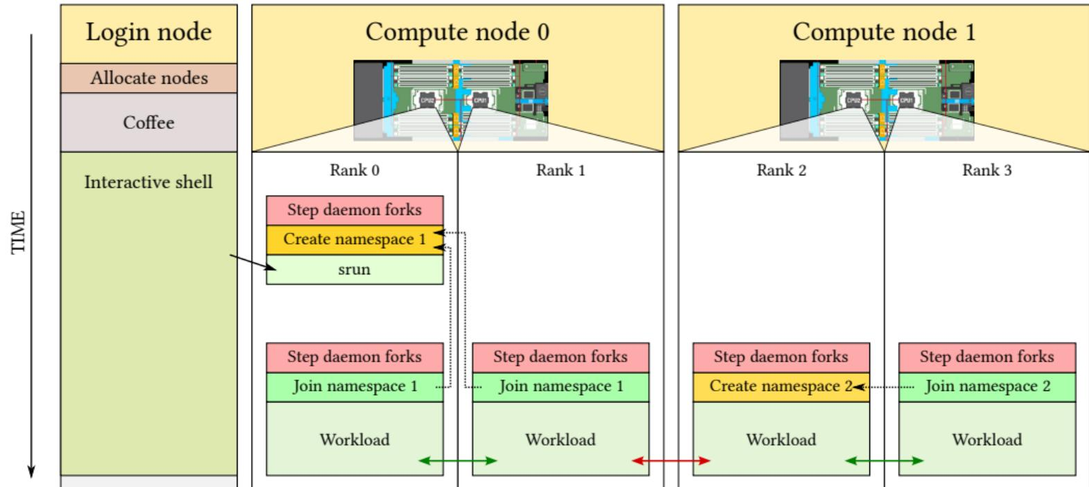
Finally, we can safely run the workload in parallel using **one** user namespace per node.
